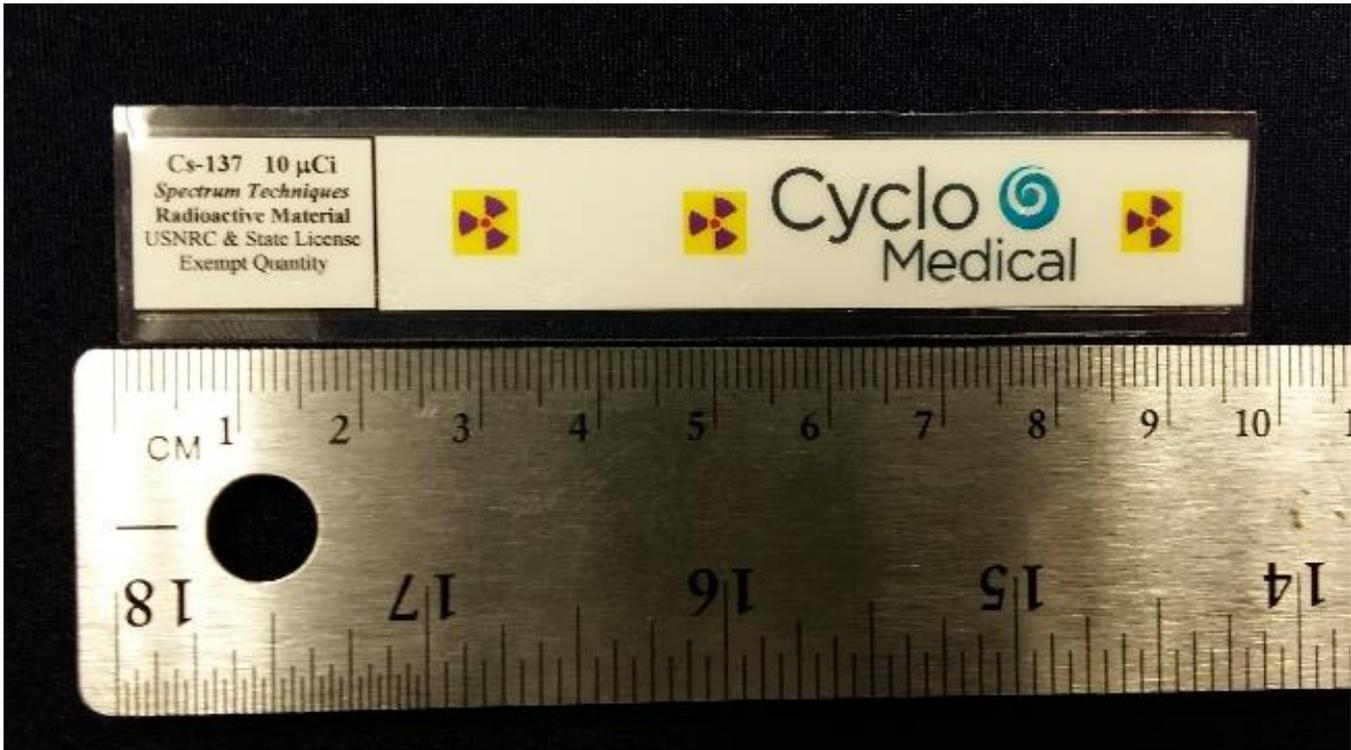
**Figure 1. Picture of RTL Daily Check Source Strip. Distances of red dots (point sources of activity) are 1cm, 5cm, and 7cm (+/- 0.05cm) from the right side of the strip of paper.**
